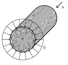
Temperature will be treated as a passive scalar under isoflux (constant heat flux) conditions, and the Nusselt number will be evaluated for all cases and compared with the azimuthally homogeneous case as well as literature correlations, such as the Gnielinski correlation. Select cases will also be simulated for liquid metals, which are characterized by a larger characteristic length scale of heat transfer compared to turbulence, resulting in a lower Prandtl number.
